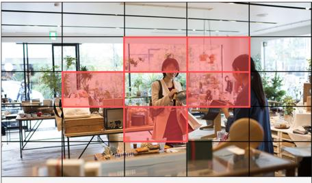
In the selected area, alarm and video recording will occur when the object is detected to move. in the horizontal screen mode, the area selection is more convenient
