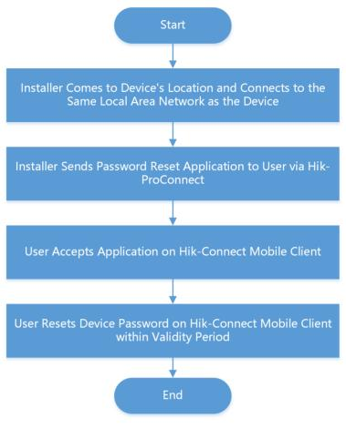
Figure 4-4 Flow Chart of Resetting Device Password
